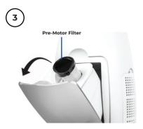
Remove the Pre-Motor Filter by grasping the Pre-Motor Filter handle and turn counter-clockwise to the unlock position. Pull Pre-Motor Filter straight up and out of the top of the Canister.
