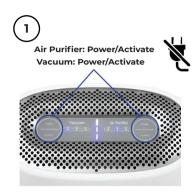
Starting with the vacuum side, touch the Power button, and cycle to the off position. On the air purifier side, touch the Power button and cycle to the off position. Then, unplug the EyeVac Air.
