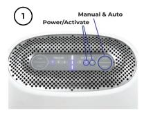
Touch Power button to turn EyeVac Air on in Manual mode. Touch Power button again to select Auto mode. A blue LED indicates the unit is on. Long press Power button for 2 seconds to run the air purifier permanently.
